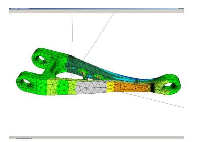
With the Displacement Scale set to '1', this represents the actual deformation that the part will experience under this load, which tells us that we may want to use a different material or a different design, or change the operating environment for this part.
