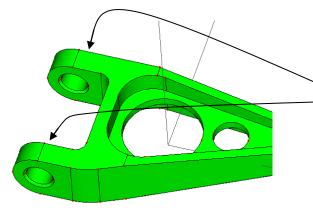
From our current view, let's say we want to fix the faces of the two axially aligned holes that are facing away from us.
