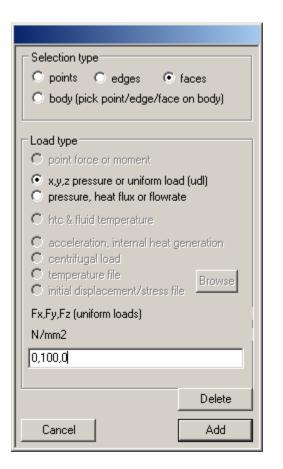
For our mechanical elastic analysis, "Selection type" should be 'faces' and "Load type" should be 'x,y,z pressure or uniform load (udl)'.
