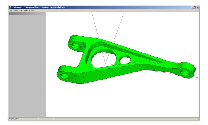
**View manipulation:** To obtain a better view of the part, dynamically rotate on screen by holding the right mouse button down and moving to rotate the view to the desired perspective. Zooming is done by simply drawing a window around the whole part, or the area of the part that you want to examine more closely. To quickly zoom out to see the entire model on screen, simply single-click anywhere in the model window.
