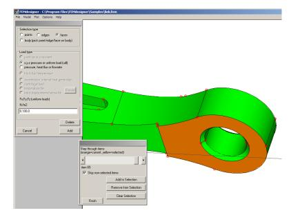
When you have the selection set to the single face shown at left, click the 'Add' button in the Load dialog to apply the load to this face. Selecting 'Cancel' dismisses the dialog box, but retains any loads you have applied.
