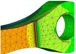
As one would expect for this analysis, the highest stresses occur at the thinnest cross-sections of the part, and maximum stress occurs on this thin cross-section at the sharp corner that is transverse to the direction of the applied load, shown at left.
